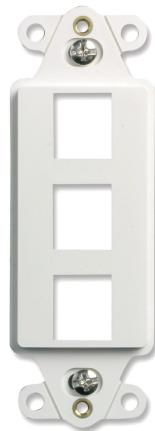
The non-flexing design of the On-Q Decorator Outlet Strap provides security when plugging and unplugging cables. Steel threaded inserts with recessed hex design to reduce spin for faceplate mounting and easy leveling to compensate for off-center boxes.
