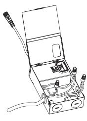
**6.** Place all wiring and connections back into the box and close the cover.
