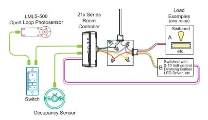
Plug DLM local network components together in any configuration using Cat 5e cables with RJ45 connectors.
