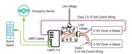
Plug DLM local network components together in any configuration using Cat 5e cables with RJ45 connectors.
