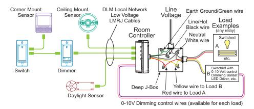
Plug DLM local network components together in any configuration using Cat 5e cables with RJ45 connectors.
