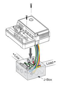
box. Depending on outputs used, an extension box may be needed. Connect to single 20A (120 or 277V) circuit.
