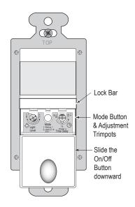
25' (7.6m) To access adjustment dial, gently pull the lock bar away from the switch face and slide the on/off button down.
