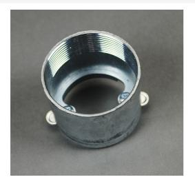
Installed either before or after concrete pour to create activation from duct. NOTE: Drill a 2 1/2" (64mm) hole in concrete and a 2 1/4" (57mm) hole in duct.
