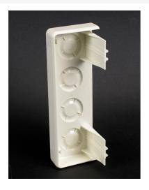
Closes off end runs of 5400 Series Raceway. Has four 1/2" trade size KOs for end feed.
