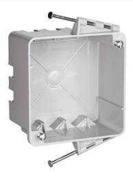
4-inch Square Box with Threaded Mounting Holes, captive Mounting Nail each end. Three Auto/Clamps each end, Two on side adjacent to nails. Two #8 mounting screws factory installed.
