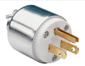
Armor Plug Grounding in white with two poles and three wires. Its rugged nylon construction provides impact and chemical resistance. All 3-wire terminals are located on the same plane, allowing for quick wire termination from any angle. 15A, 125V.
