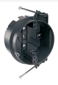
4\\ Round Ceiling Box with two captive mounting nails and four Auto/Clamps. It is constructed of impact-resistant Noryl thermoplastic, making it virtually unbreakable and non-conductive. Its depth-mounting gauge at bottom of bracket helps you align the box at the proper depth relative to the ceiling. 50 pack.
